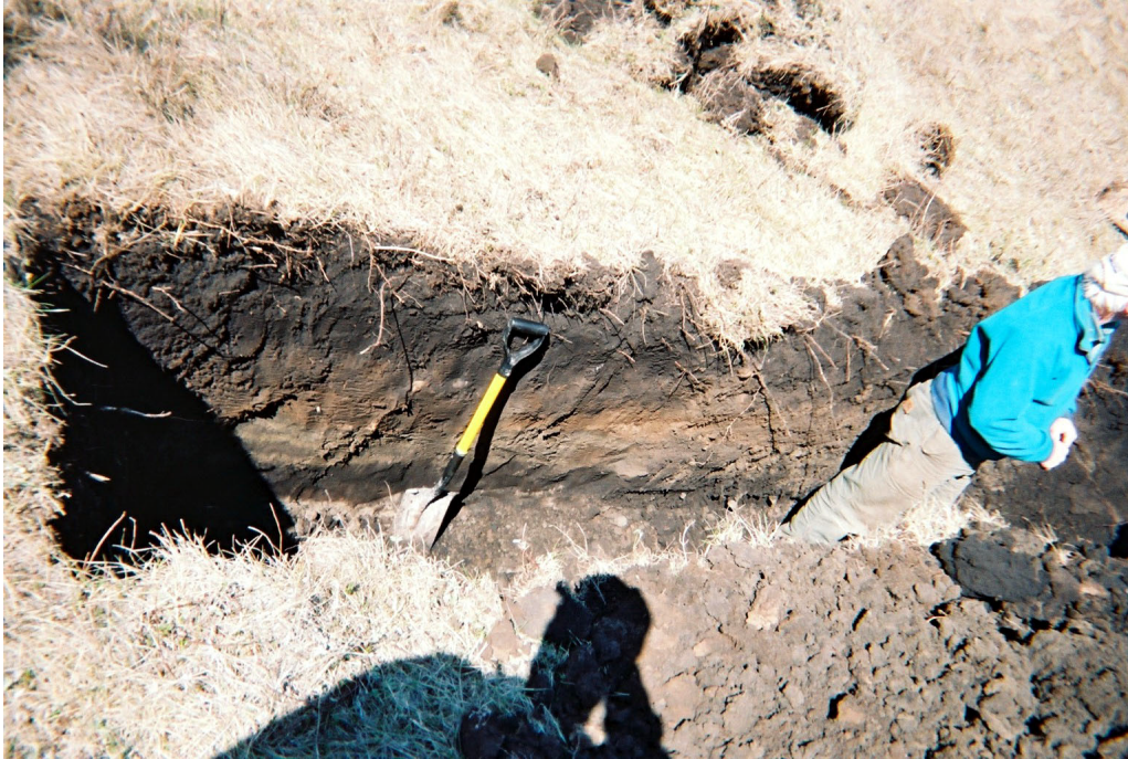
Plate 6. Backhoe Test #2, Stratigraphic Profile
