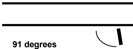
Figure 1 - Horizontal Angling of Sign Face
