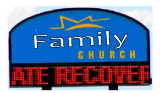
An electronic changeable copy sign is defined as a sign or portion thereof that displays electronic, non-pictorial, text information in which each alphanumeric character, graphic or symbol is defined by a small number of matrix elements using different combinations of light-emitting diodes (LEDs), fibre optics, lightbulbs or other illumination devices within the display area.
