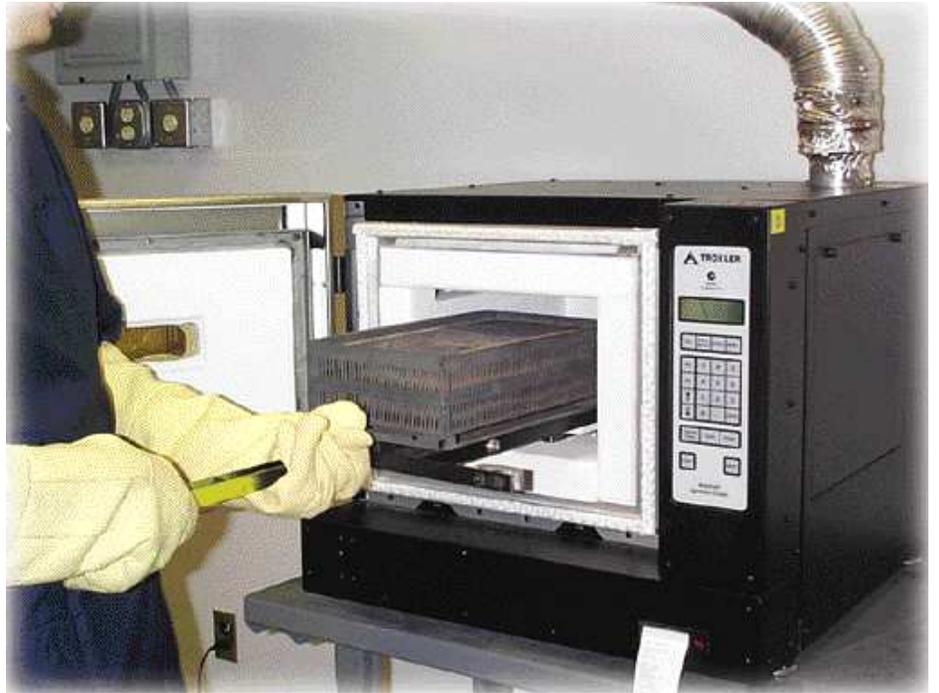
FIGURE 3-4 Troxler Ignition Oven
