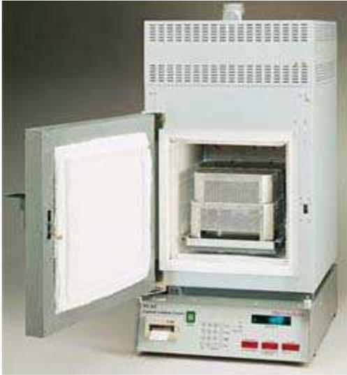
FIGURE 3-3 NCAT Ignition Oven
