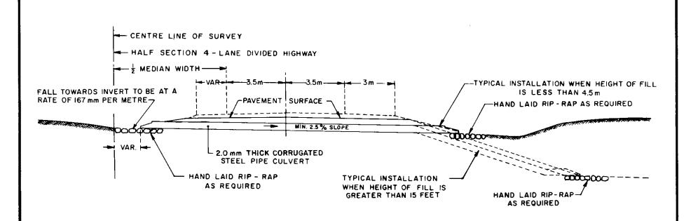
NOTE: DURING SUBGRADE CONSTRUCTION, A MINIMUM OF 0.3 METRE OF COVER IS TO BE PROVIDED AND MAINTAINED OVER THE CORRUGATED METAL PIPE CULVERT TO PROTECT THE STRUCTURE FROM DAMAGE.
