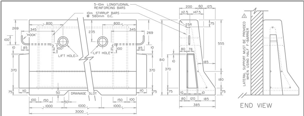
NOTE: LIFT HOLES SHALL HAVE 80mm INSIDE DIAMETRE AND AN IIOmm OUTSIDE DIAMETRE.
