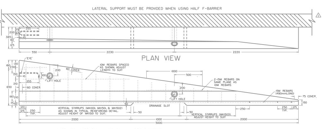
NOTE: LIFT HOLES SHALL HAVE 80mm INSIDE DIAMETRE AND AN IIOmm OUTSIDE DIAMETRE.
