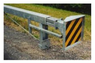
The Bursting Energy Absorbing Terminal (BEAT) system is a proprietary, energyabsorbing redirective terminal designed to shield the end of the Box Beam Barrier.
