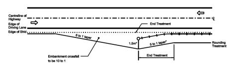
\* The 1.5m and 5:1 taper dimension are "preferred" dimensions. Refer to Standard Drawings for typical minimum dimensions.
