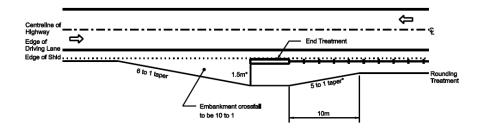
FIGURE H6.2 Minimum Grading Requirements for Gating End Treatments
