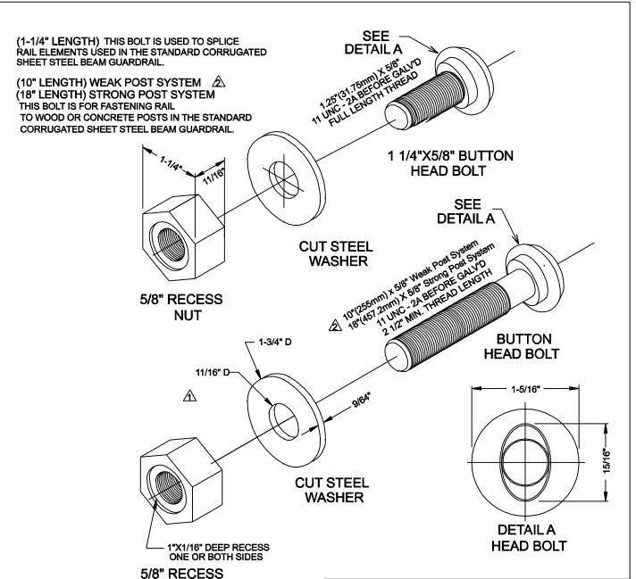
BOLTS SHALL CONFORM TO THE REQUIREMENTS OF A.S.T.M A307 AND NUTS TO THE REQUIREMENT OF A.S.T.M A563, GRADE A OR BETTER, AND BE GALVANIZED IN ACCORDANCE WITH CSA G 164-M EXCEPT WHEN CORROSION RESISTANT STEEL IS REQUESTED IN WHICH CASE BOLTS AND NUTS SHALL BE MADE OF MATERIAL HAVING AN ATMOSPHERIC CORROSION RESISTANCE, APPROXIMATELY TWO TIMES THAT OF CARBON STRUCTURAL STEEL WITH COPPER AND SHALL NOT BE GALVANIZED.
