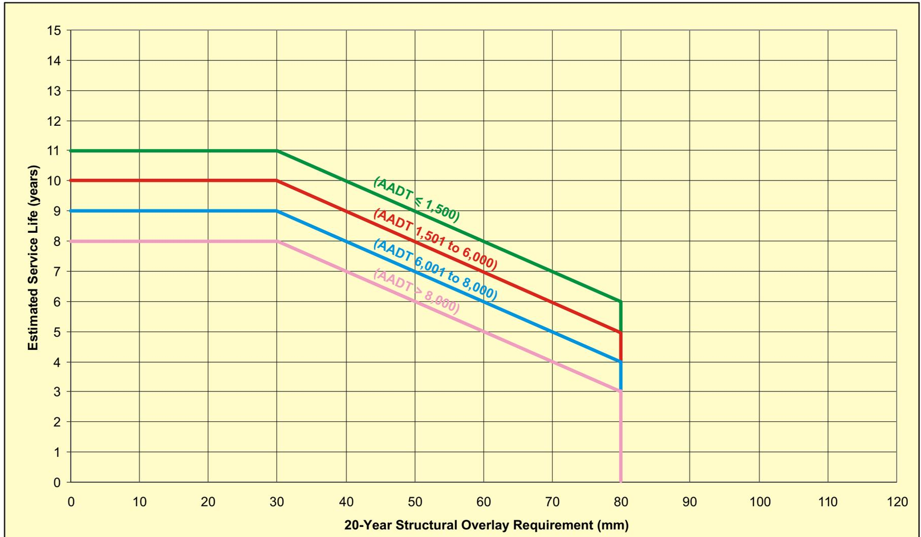
**FIGURE 6: TREATMENT MATRIX FOR TRANSVERSE CRACKS**
