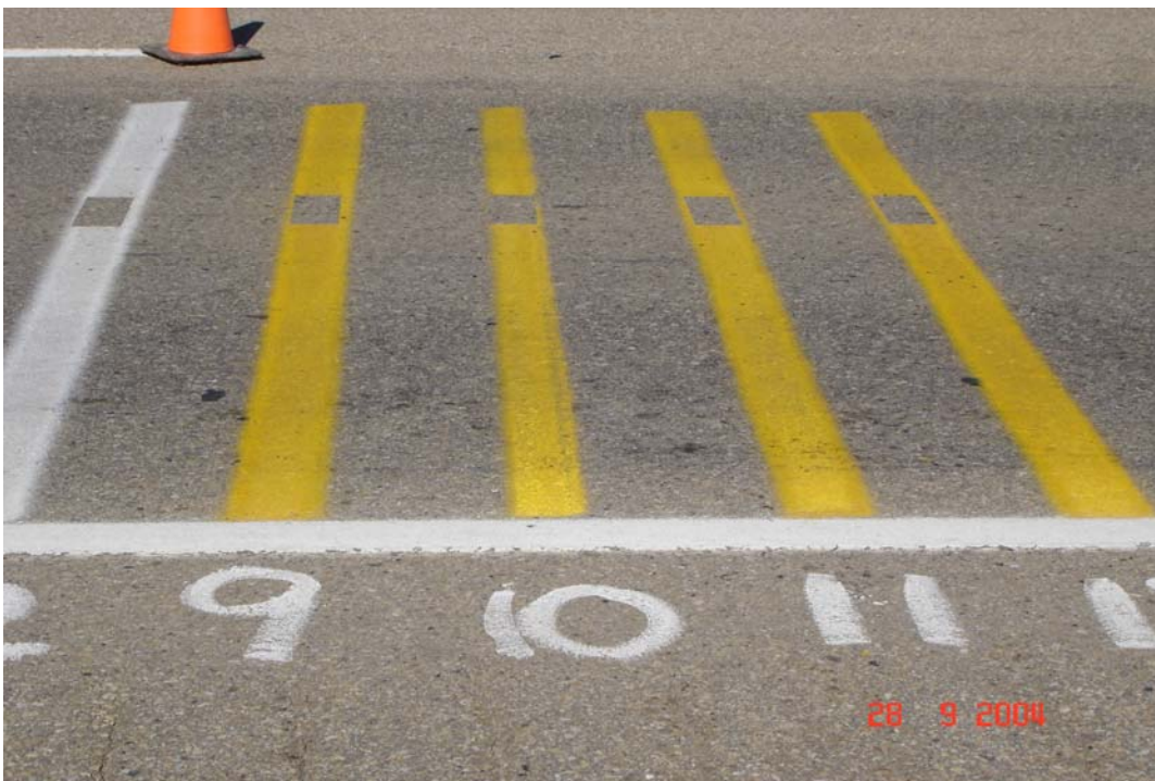
Yellow paint, line #9 – 15mil, line #10 – 12mil and line #11 – 13mil
