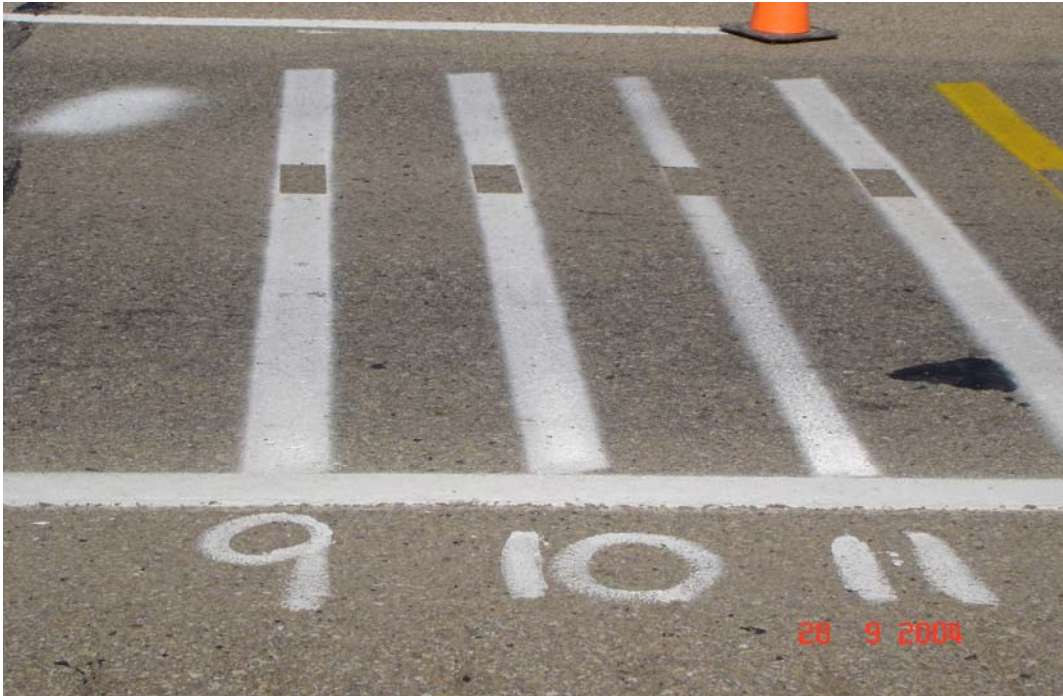
White paint, line #9 – 15mil, line #10 – 13mil and line #11 – 12mil
