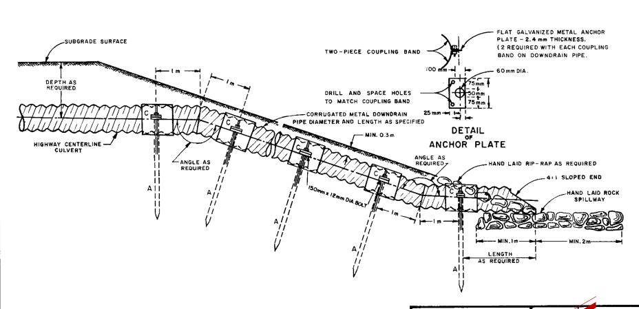
A METAL ANCHOR 40 mm STEEL PIPE OR EQUIVALENT. MIN. LENGTH 2 m MIN. WEIGHT 5.4 kg/LIN.m (2 REQUIRED FOR EACH COUPLING BAND ON DOWNDRAIN PIPE)
