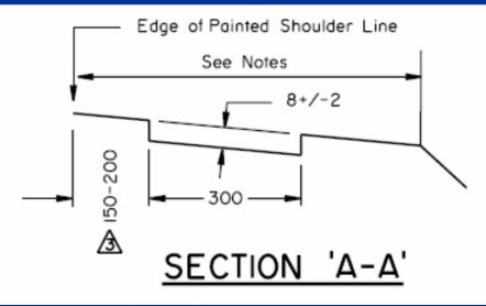
Milled-In Continuous Rumble Strips on the Inside Shoulder of a Segment of Highway 16 (Divided), West of Edmonton, Alberta (1997)
