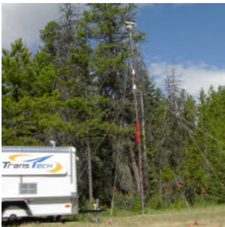
BC's infrared camera on mast
