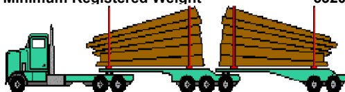
8 Axle B-Train Minimum Registered Weight 63,500 kg Other (Draw diagram of configuration if not shown)
