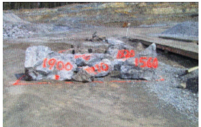
10-6 Heavy rock riprap sampled at pit with weights painted on each rock
