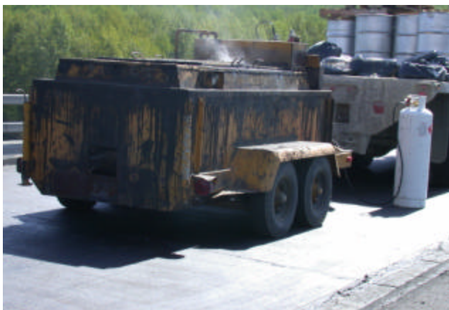
16-3 Waterproofing membrane material heater
