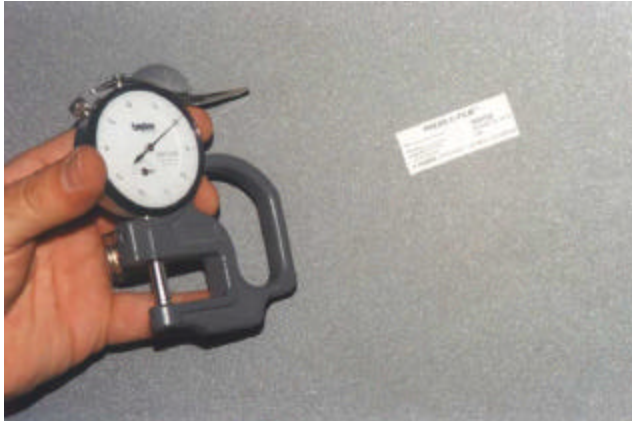
22-45 Profile meter and tape for checking anchor pattern produced by sandblasting
