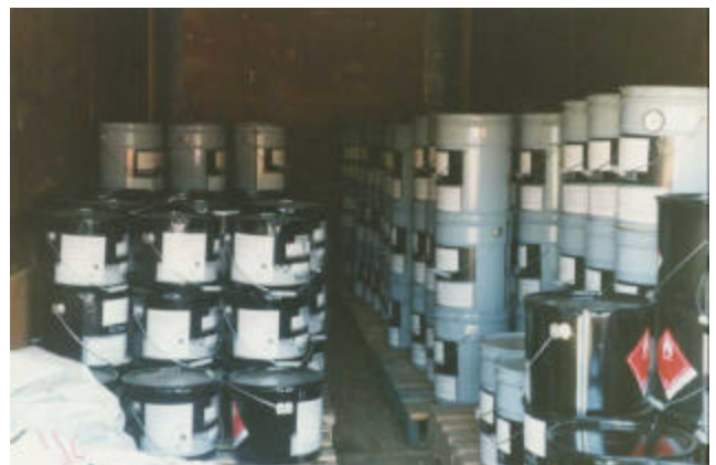
22-50 Paint storage in temperature control trailer
