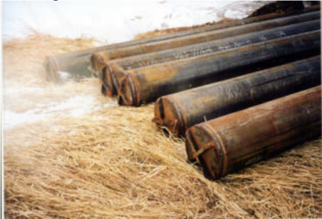
3-22 Typical closed end detail
