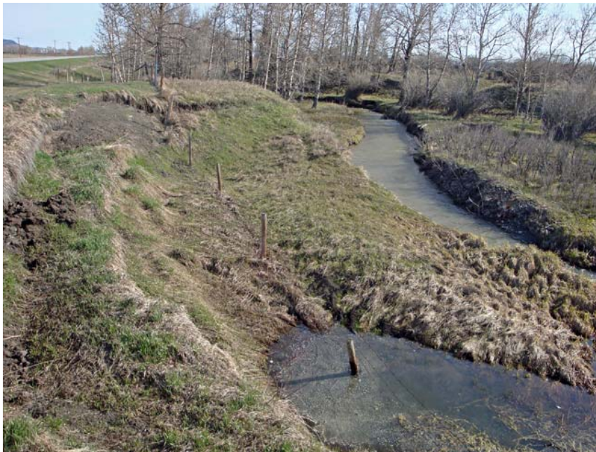
Photo S44-6 (May 2014) At Site B, standing on the east side of the highway at the south end of Slide Area B1 looking towards the northeast at the circular earth slide within the bank meander.
