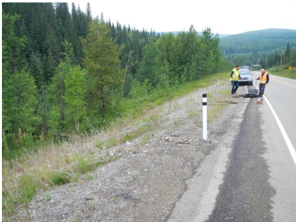
Inclinometer 2005-7 being read
