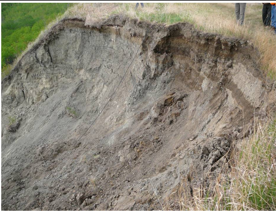
Photo 6. Further significant slide movement in the backscarp of Slide 4. Note the bands of wet soil in the backscarp.
