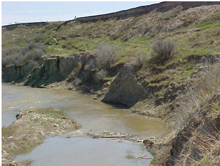
Photo 8 – Close-up of toe of central portion of slide, partially protected from direct erosion by island in creek. Note oversteepened portions of toe slope.
