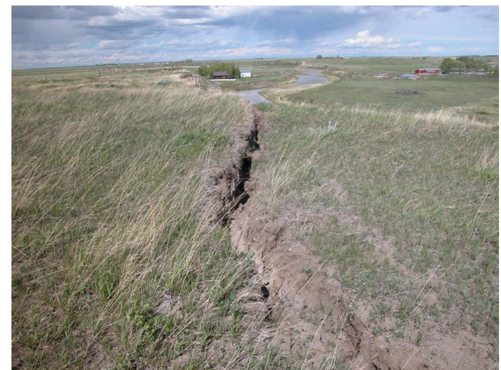
Photo S4-3 (lower left) – May 2004 – closer view of area shown in Photo S4-2. SI #8 is visible on the right hand side of the photo, just west of the fenceline. The scarp in this area retrogressed approximately 1 m between the October 2002 instrument readings and the July 2003 inspection. It does not appear that significant additional retrogression has occurred since July 2003. However, as noted in previous reports, the crest retrogression generally occurs in 0.5 to 1 m increments in response to toppling of soil blocks from the scarp, rather than a steady rate of retrogression.
