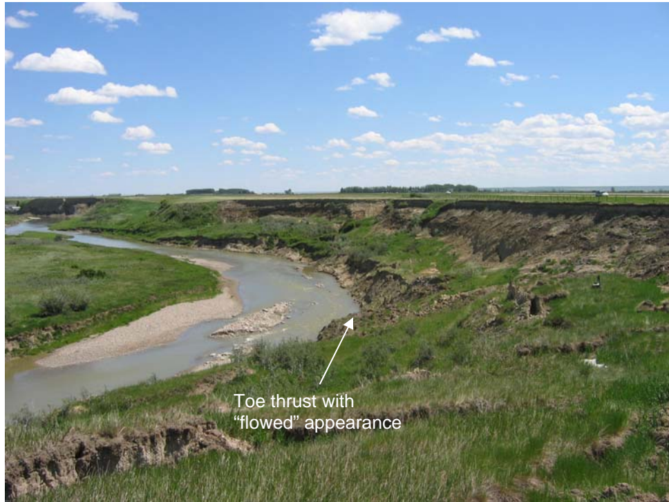
Photo S4-4 (upper left) – May 2006 – facing south across the landslide area. Note the portion of the toe of the landslide that thrust outwards into the creek channel. The material that was thrust into the creek channel had a “flowed” appearance.
