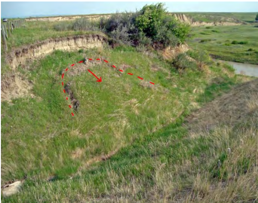
Photo S4-4 (May 2013) – Standing on the south side of the erosion gully at the south end of the site, looking towards the northeast at a recent translational slide on the north side-slope. The extents and direction of the failure are outlined in red.
