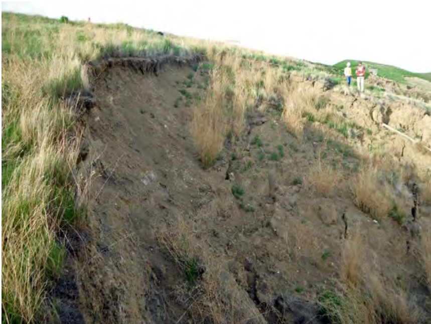
Photo S5-5 (May 2013) – Looking towards the same slide area as Photo S5-4. The exposed soil has eroded but the condition is generally unchanged.
