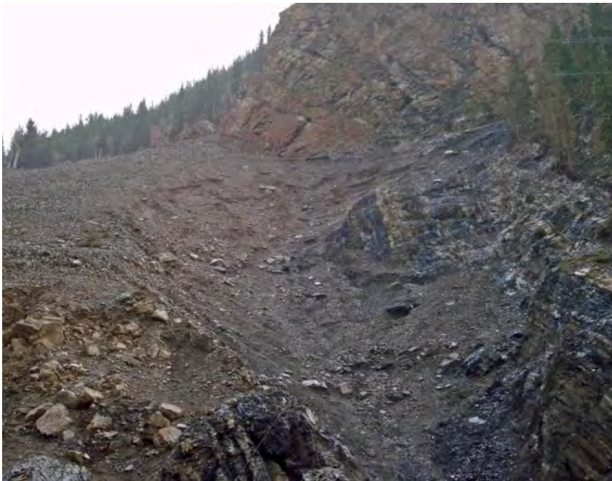
Photo S15-7 (May 2013) – The upper gully in the talus slope as observed during the 2013 inspection. The gully has continued to expand toward the cliff face. Several of the larger boulders visible in 2012 have since fallen.
