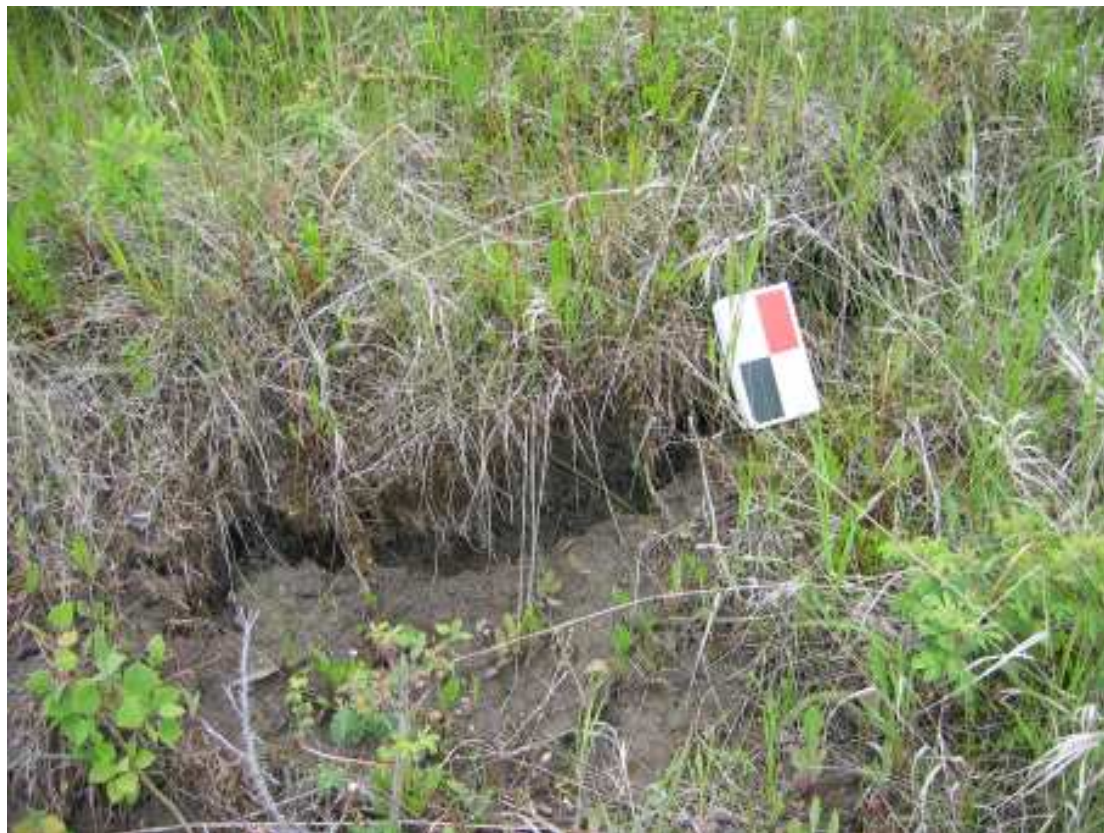
Photo S3-2 (lower left) – June 2005 – tension crack showing recent movement around the north flank of the slope movement shown in Photo S3-1. Field notebook for scale.
