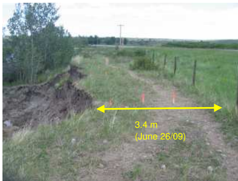
Photo 4 (bottom) – View north along the slope crest, at the point of maximum retrogression towards the highway (offset 3.4 m from the fenceline). Reference stakes were placed at selected locations along the slope crest, at 0 and 1 m offset along with a third stake at 2 m offset at the location shown.
