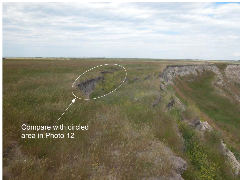
Photo 11 (lower left) – July 2003 Facing northeast across new landslide block forming near SI #10, as seen during the July 2003 inspection. Compare with Photo 12 of the same area, from the May 2002 inspection, and note the increased displacement and downdropping of the landslide block over the past year.
