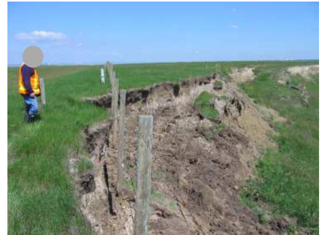
Photo S4-2 (upper right) – June 2005 – facing across the area where the landslide scarp has retrogressed across the fenceline since the 2004 inspection.
