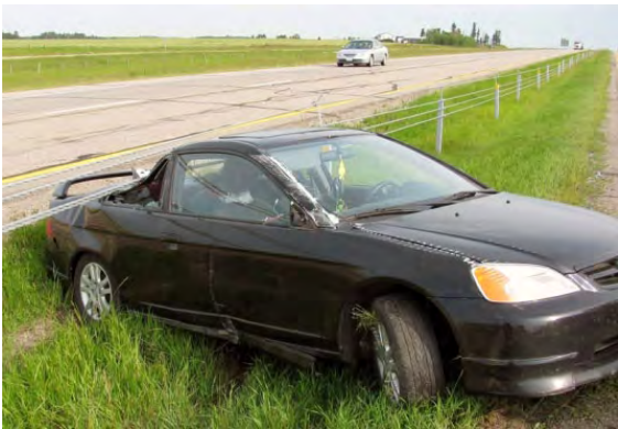
High tension cable barrier prevents this vehicle from going into oncoming traffic
