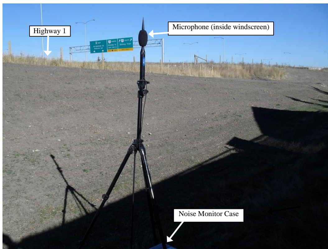
Figure 5. Noise Monitor at Location 4
