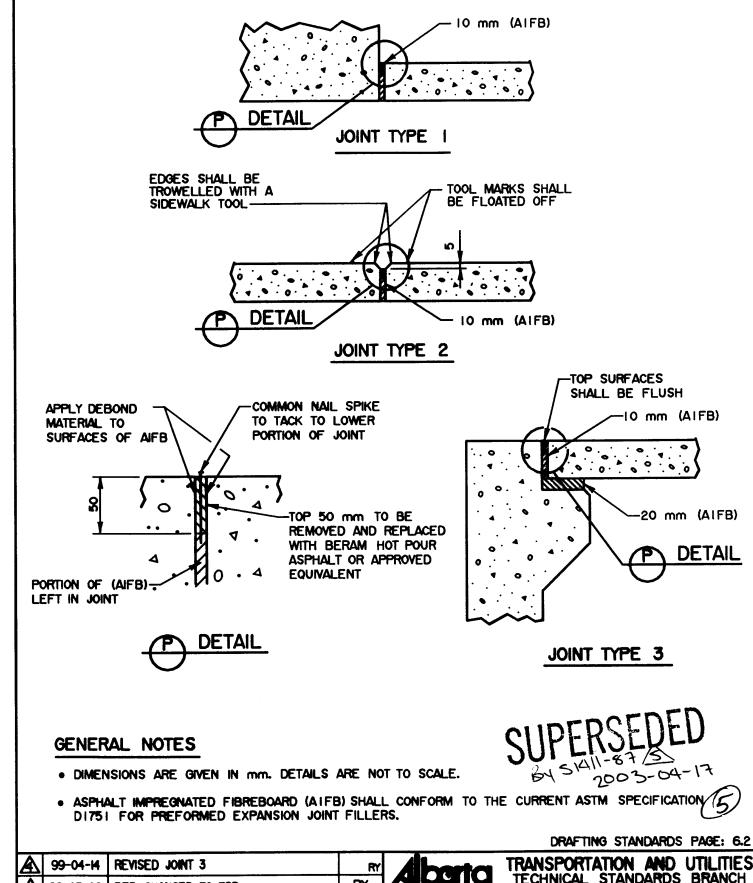
ASPHALT IMPREGNATED FIBREBOARD (A I FB) SHALL CONFORM TO THE CURRENT ASTM SPECIFICATION (5)
