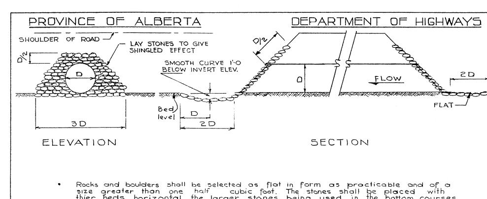
Rocks and boulders shall be selected as flat in form as practicable and of a size greater than one half cubic foot. The stones shall be placed with thier beds horizontal, the larger stones being used in the bottom courses and the smaller stones at the top.
