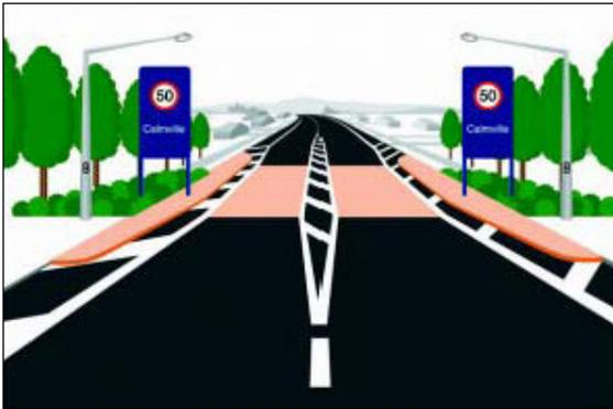
FIGURE 3.8 ILLUMINATION, SURFACE TREATMENT, ROADSIDE VERTICAL ELEMENTS, PHYSICAL AND VISUAL ROAD NARROWING<sup>29</sup> (NEW ZEALAND)
