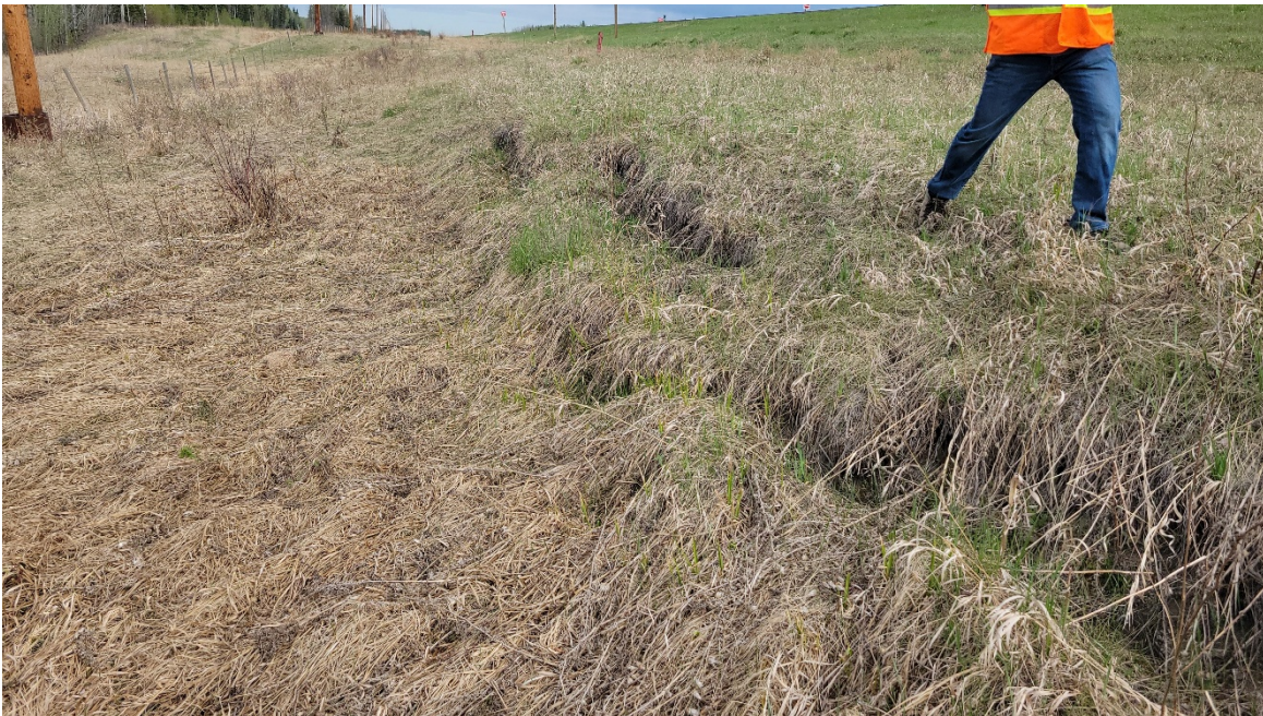
Photo 2. Looking north at slide backscarp crack (300 mm wide, up to 200 mm deep).
