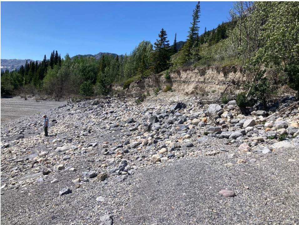
Photo 10 The eroding slope along the C034-3 is approximately 110 m long and 3 m to 4 m tall. Photo taken June 9, 2025 facing west.
