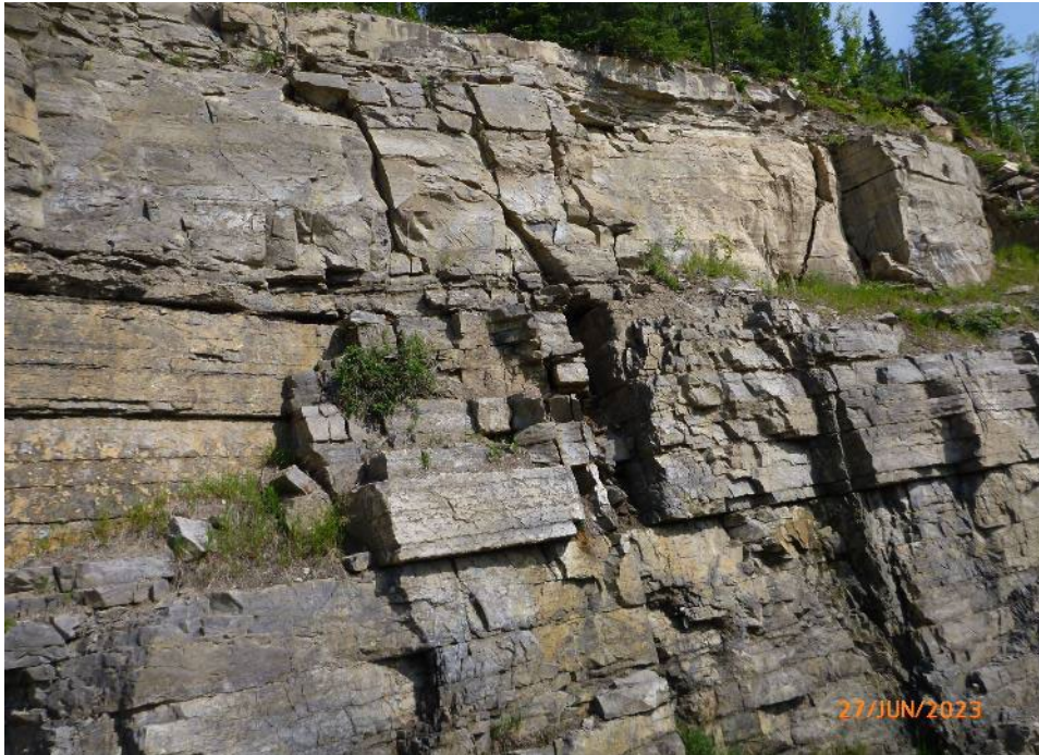
Photo 6 The relatively intact rock slope along the middle and west portion of the site. There is a potentially unstable shelf of rock at the top of the rock slope (indicated by red arrow). Photo taken June 27, 2023, facing north-northeast.
