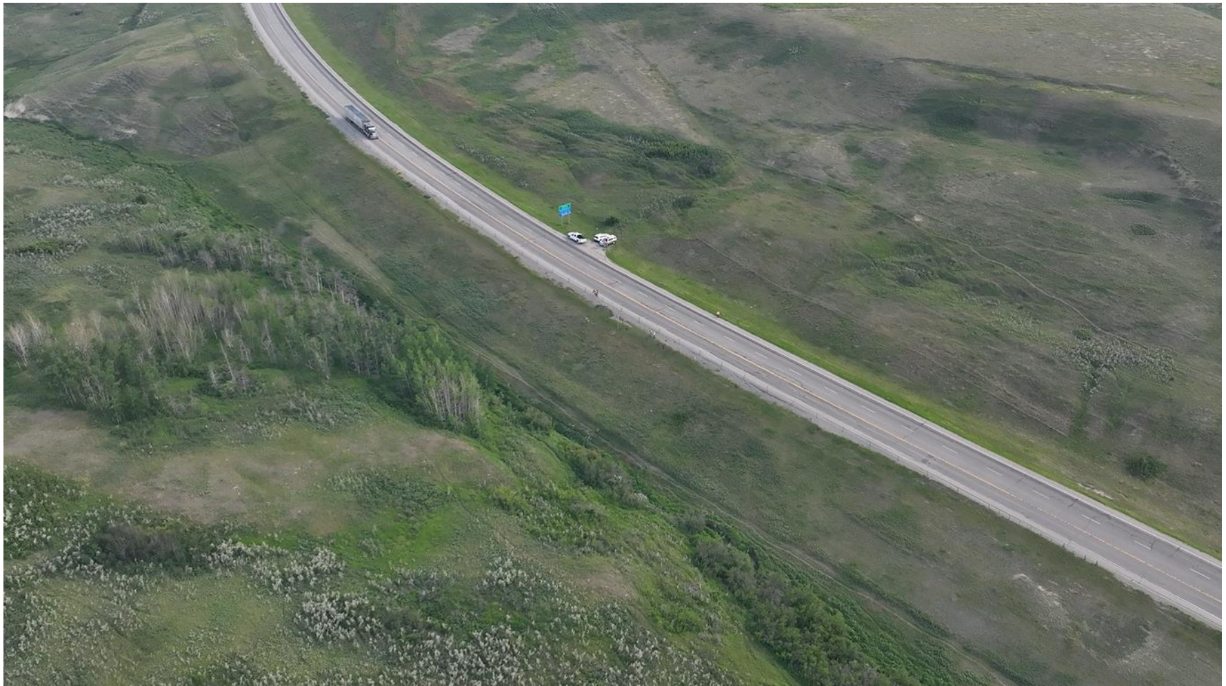
Photo 5 Aerial photo of C067 Site B located downslope (southeast) of Site A. The highway embankment slope is well vegetated and generally even, indicating the H-pile wall is performing well. Photo taken June 10, 2025 facing north-northwest.
