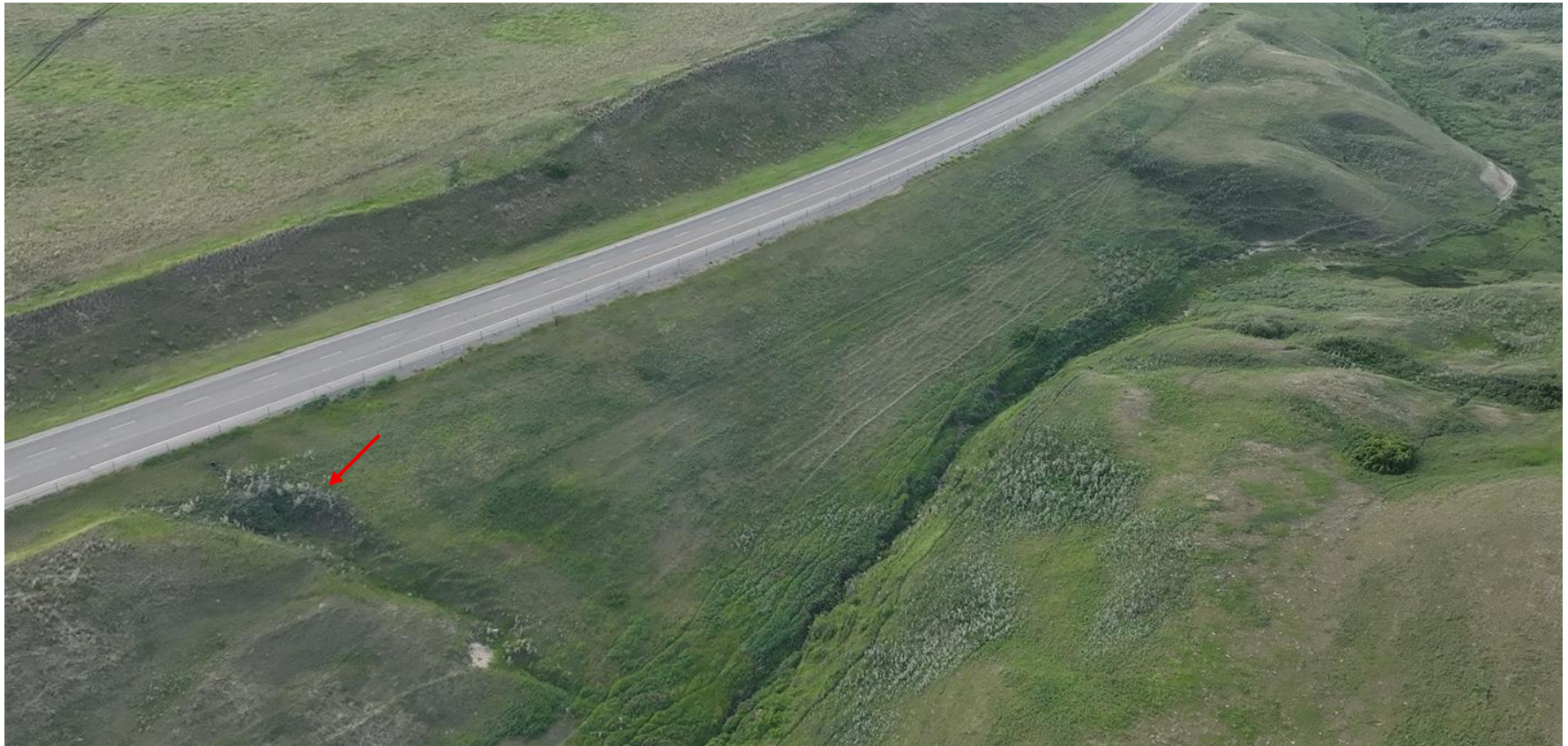
Photo 2 Aerial photo of the C067 Site A upslope (northwest) of Site B. The highway embankment slope is well vegetated, no pavement distress attributed to slide movement was observed, and an erosion gully is at the north extent of the site (indicated by red arrow). Photo taken June 10, 2025 facing southeast.
