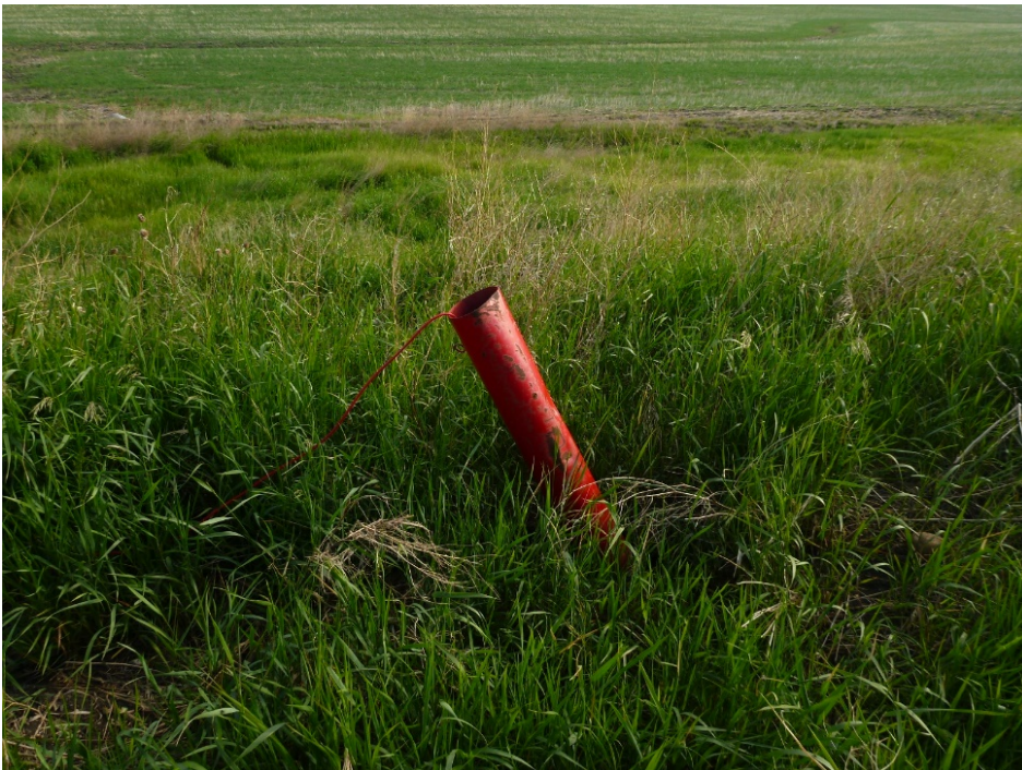
Photo 2 View of the destroyed VWP and SI that was installed in March 2017 at C070E. Photo taken June 13, 2018 looking north.
