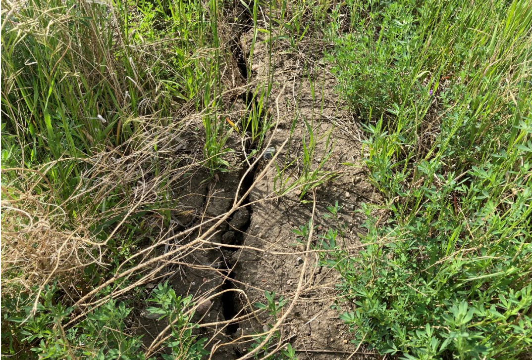
Photo 4 Location of ground cracking observed southwest of Waypoint 711 near the power poles at the top of the slope. Photo taken June 24, 2020 facing north.
