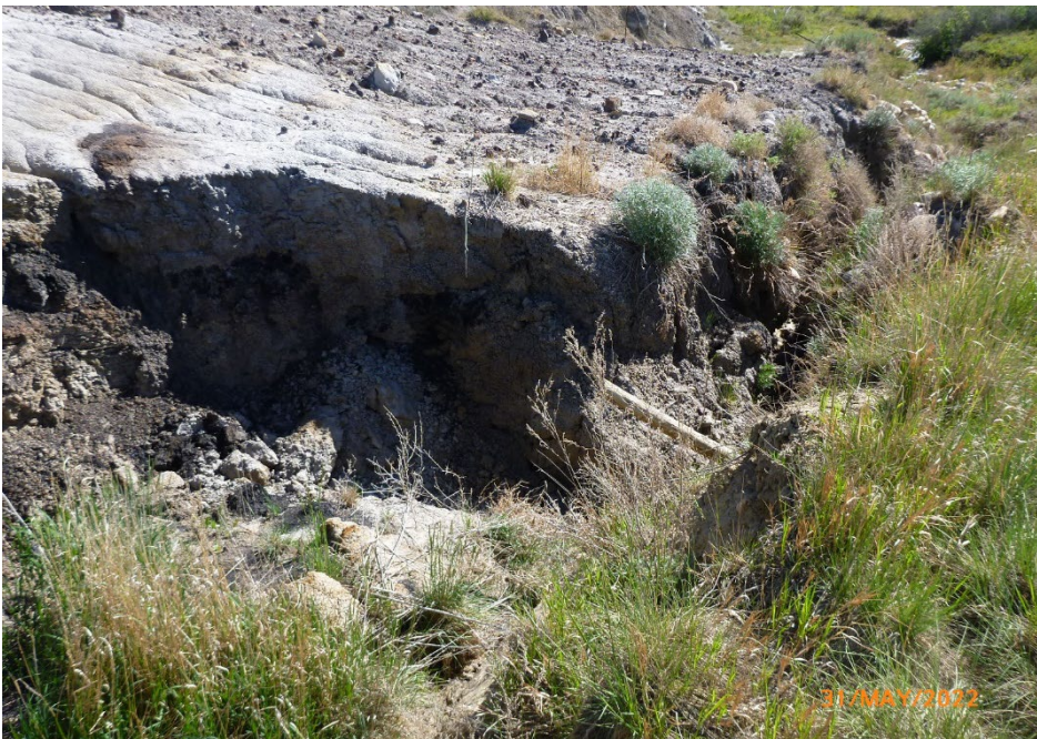
Photo 5 Potential coal-mine sinkhole first observed during the 2021 inspection, located at Waypoint 166. Photo take on June 24, 2021, facing northeast.
