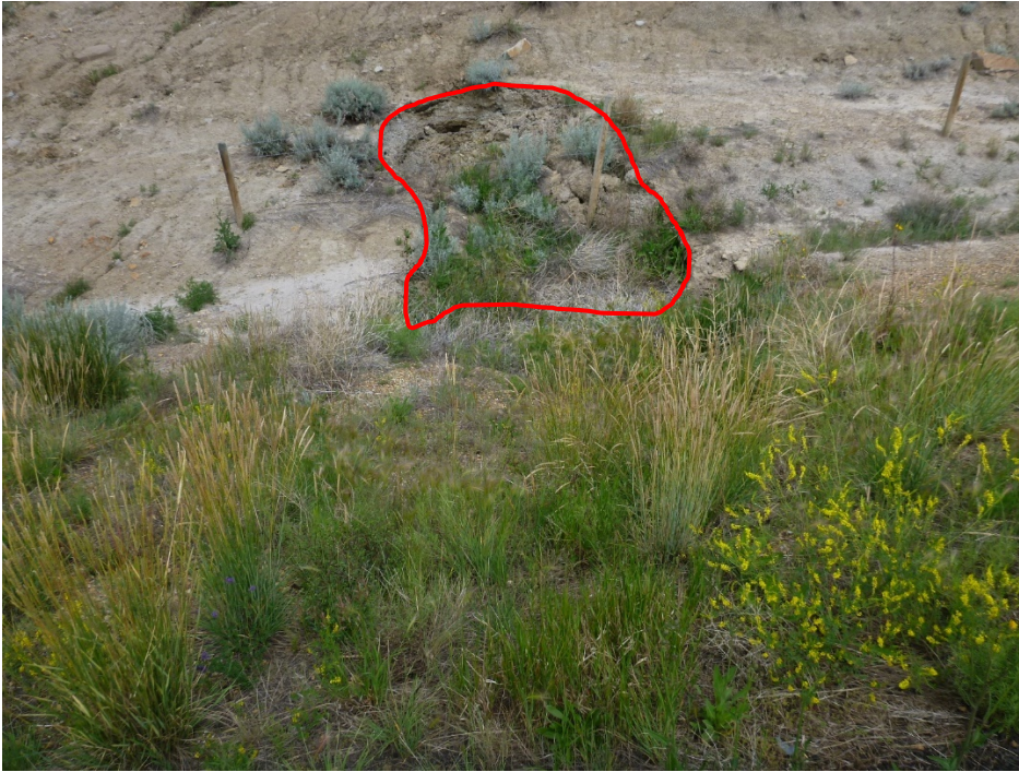
Photo 4 Small sinkholes along the south side of the highway near the fence line at C055-II, west of the culvert outlet (waypoint 22). Photo taken July 10, 2019 looking southeast.
