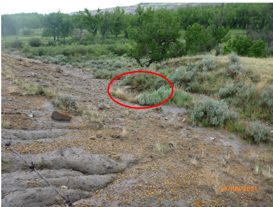
Photo 6 Large sinkhole (indicated by a red circle) at the toe of the south slope below highway at C058-III has not expanded since 2019 inspection. Photo taken June 24, 2021 looking southeast.
