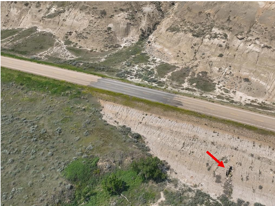
Photo 12 Aerial photo of the C058-3 site showing the pavement patch and culvert outlet (indicated by red circle). Photo taken June 10, 2025 facing north.
