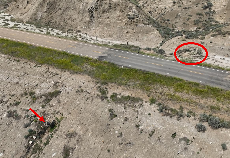
Photo 12 Aerial photo of the C058-3 site showing the pavement patch and culvert outlet (indicated by red circle). Photo taken June 10, 2025 facing north.
