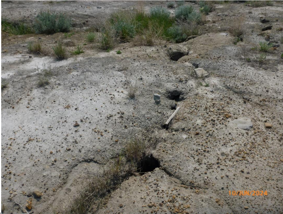
Photo 7 Sinkholes observed on the south side of the highway downslope of the site in an area of shallow bedrock. Photo taken June 10, 2025 facing south.
