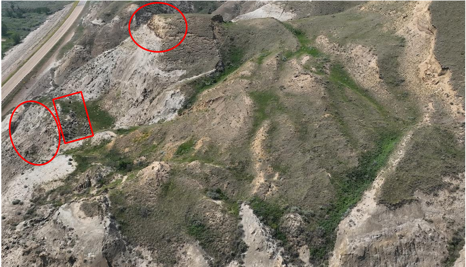
Photo 4 Aerial photo of the upper portion of the slope. Area where ground cracks have been observed indicated by red rectangle and areas previously scaled in 2022 are indicated by red circles. Photo taken June 10, 2025 facing west.
