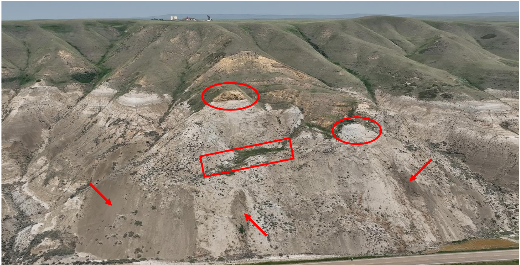
Photo 1 Aerial photo of the C077 site. Locations of recent movement are indicated by red arrows, location of cracking observed on the slope is indicated by red rectangle, and previous scaling completed in 2022 is indicated by red circles (note the area of ground cracking was also scaled in 2022). Photo taken June 10, 2025 facing north.
