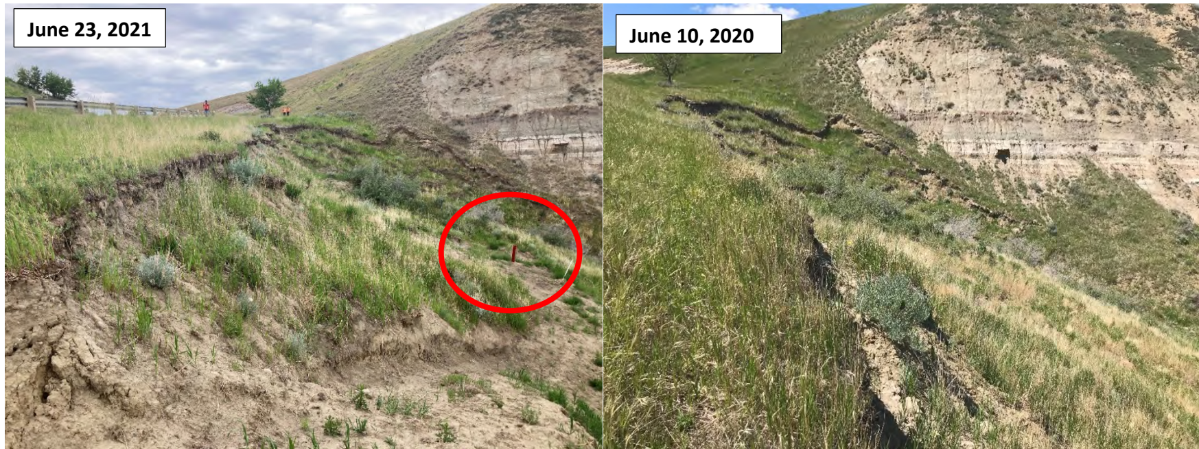
Photo 3 Comparison of the C017-III head-scarp in 2020 and 2021. The slight appears to be relatively inactive since 2020. Instrumentation installed in October 2020 are indicated by black circle. Photos taken looking east.
