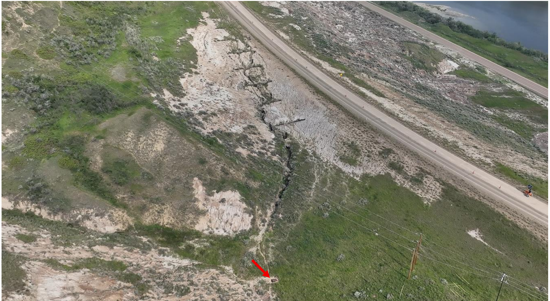
Photo 5 Aerial photo showing the lower (east) extent of the C017-2 site where the ditch grade increases to between approximately 15% and 20%. Inlet of culvert underlying Hwy 575:04 indicated by red arrow. Photo taken June 10, 2025 facing northwest.
